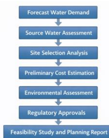
Figure 2: Water Treatment Plant Planning Process Flowchart
